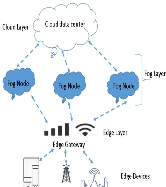
Figure 7- Fog Layer architecture
