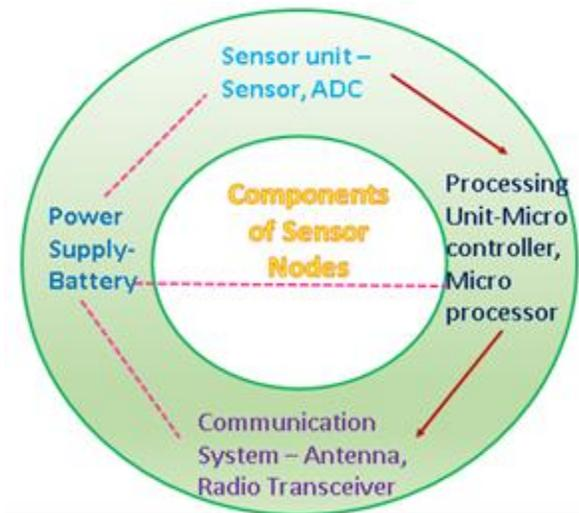
Figur3 –Sensor nodes components
